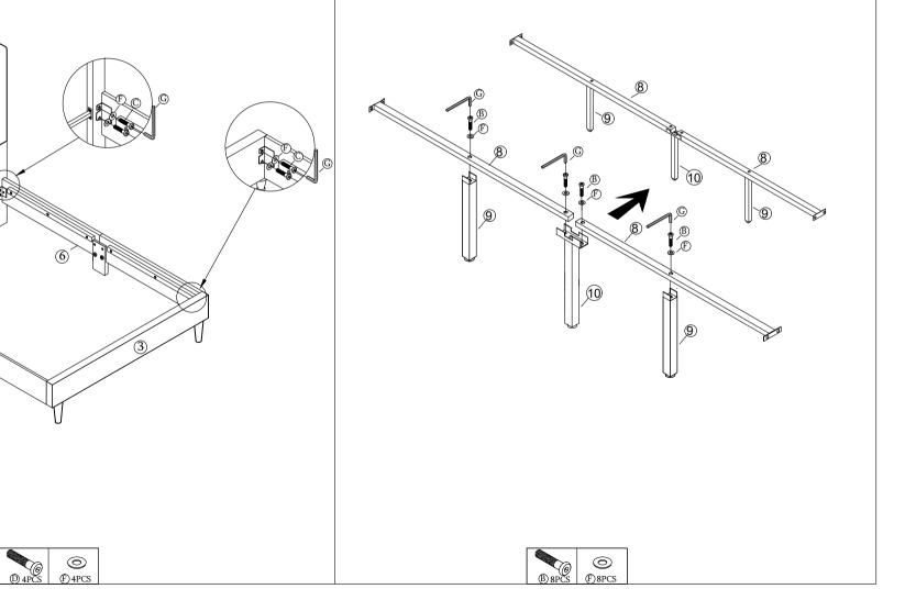
STEP 8: Take the center support rail from Step 7 and lay it in the middle of the bed from headboard to footboard. You will need 4 Part B 8 Part F and 4 Part E. Follow the diagram and bolt everything on from the center support rail to the HB cross brand (Bellow the headboard)
