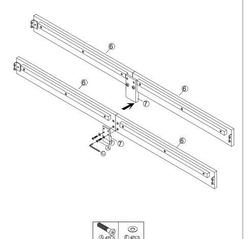
STEP 5: First, lock in your side rail and the footboard in (Look at photo). You will now take one side of the completed Side Rail and bolt that onto the Headboard, make sure the inside of the side rail is facing inside, another way to know it is facing inside is that the Side Rail feet should be on the inside of the bed. For this step you will need 4 Part C and 4 Part F.
